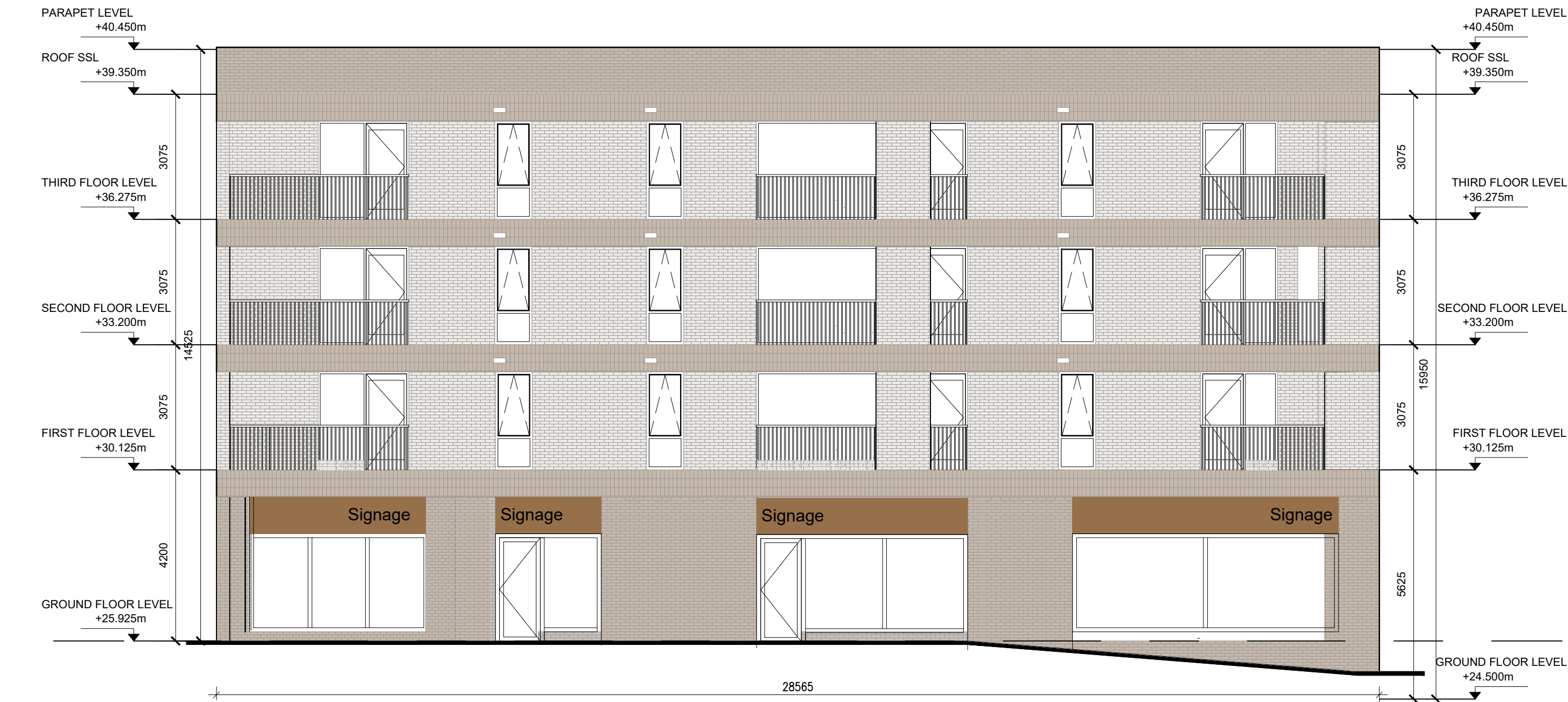
3 Block A - Proposed South Elevation 6304 1:100
