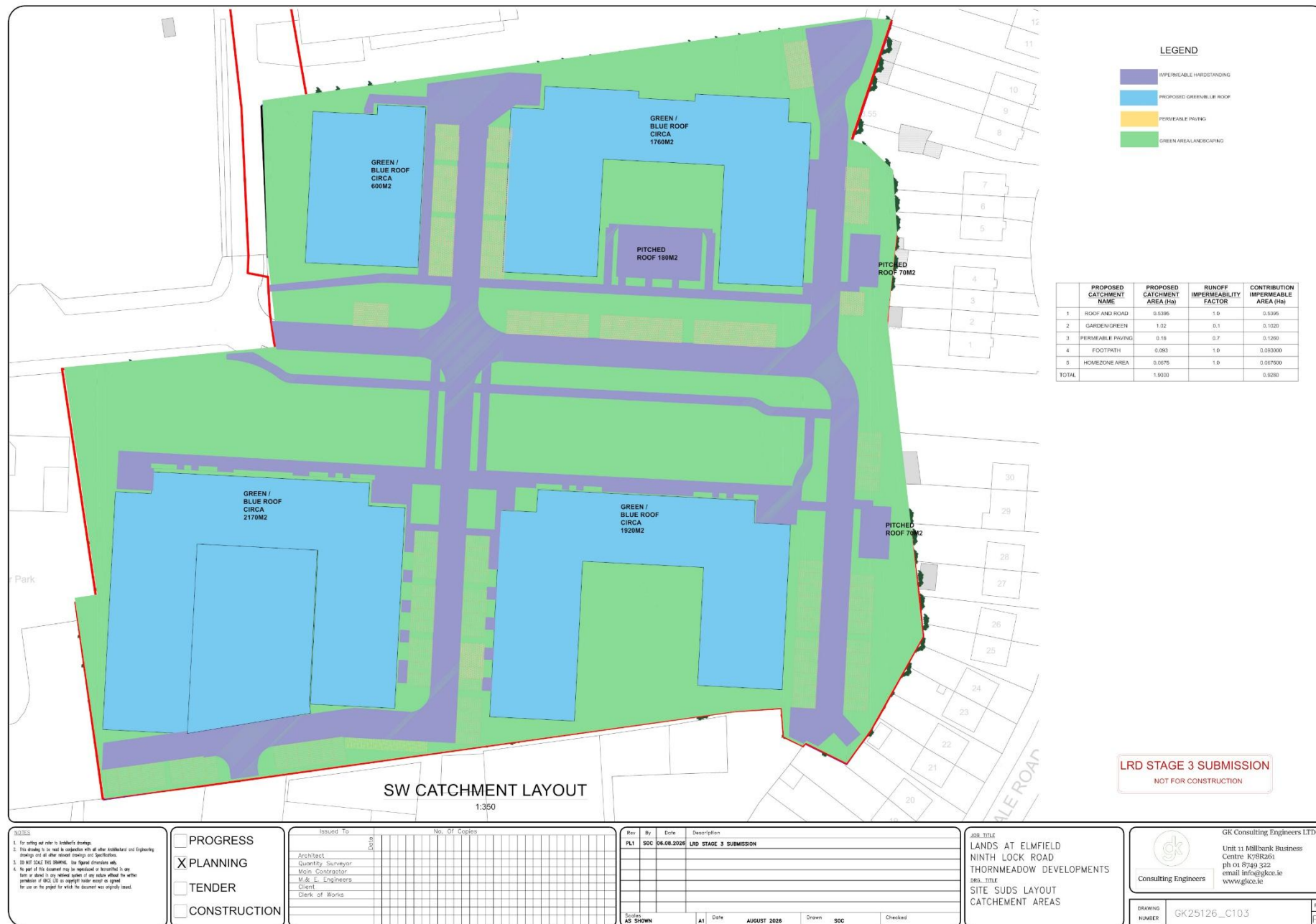
Figure 10. Proposed site SUDS layout catchment areas
